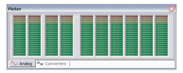
The **Meter Window** provides two tabbed views of all input and output levels of a Live device. The Analog tab shows the calculated level, in dBu, at each analog input and output.
